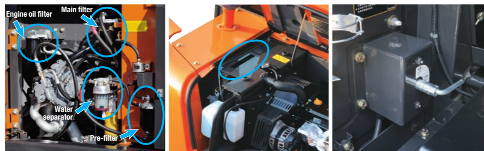
Grouped remote filters and inspection points
