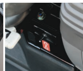
Emergency engine stop switch
